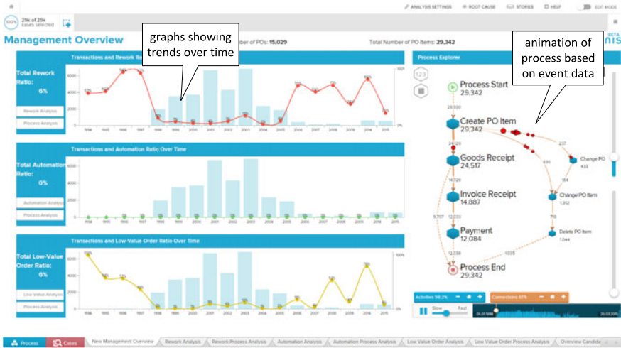
Fig. 11.13 Animation of the process obtained by replaying the event data on a simplified process model and three charts showing trends in the event data
